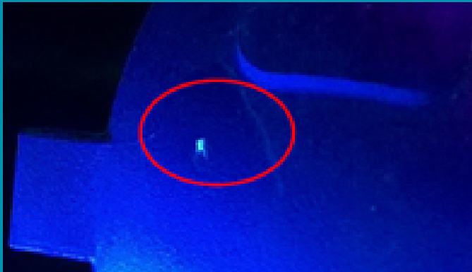
Identification of linear or non-linear indications on the surface - PT analysis
