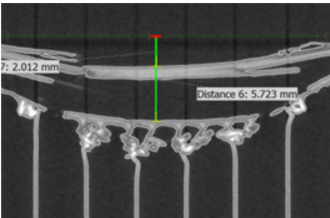
Damage depth analysis after impact by tomographic volume post processing
