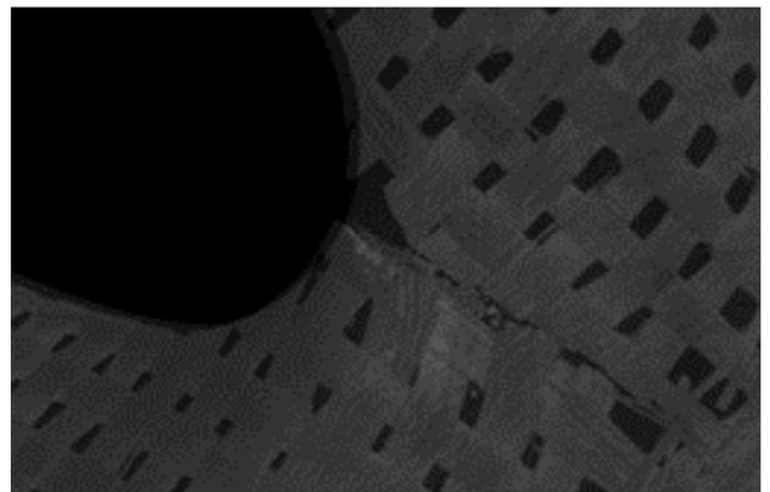
Glass fiber and carbon fiber. Fracture propagation through the fibers
