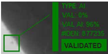
Fig. 2. When the AI system recognizes a defect, it must be validated by a human operator.
